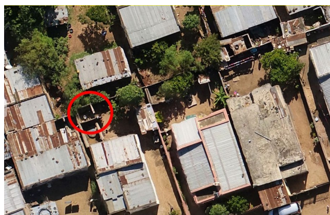
Figure 3. Drone image showing housing and sanitary conditions. In the centre left of the image a red circle highlights the presence of a latrine, without a roof. In this case a WC was installed on top of the open pit latrine.
